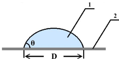
Figure 1. The sessile drop (1), the substrate (2), the wetting (contact) angle  $\theta$ , and the drop diameter  $D$ .
