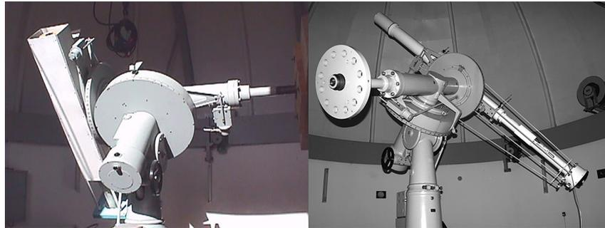
Figure 1. The first two telescopes located at the solar tower in the Bulgarian National Observatory: 13-cm refractor from the beginning of the 1990s (left) and 15-cm coronagraph from 2005 (right).
