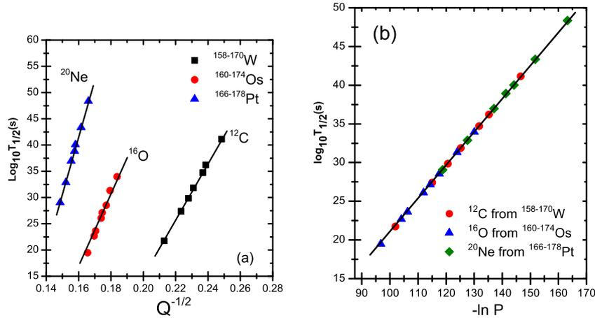
Figure 3. (Color online) (a) Geiger-Nuttall plot of half-lives vs.  $Q^{-1/2}$  for various clusters from W, Os, and Pt isotopes. (b) Universal curve for calculated  $\log_{10} T_{1/2}$  (in s) vs. negative logarithm of penetrability ( $-\ln P$ ) for alpha-like clusters ( $^{12}\text{C}$ ,  $^{16}\text{O}$ , and  $^{20}\text{Ne}$ ) decay from different parent nuclei.
