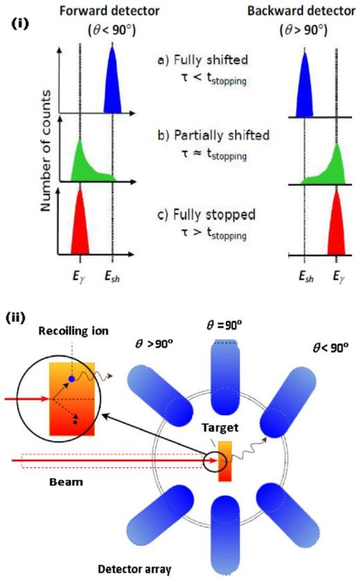
Figure 1. (Color online) (i) Position and shape of the  $\gamma$ -ray peak decaying from a nuclear state with lifetime in three different ranges, when compared with the stopping time of moving recoils in a medium. (ii) A typical arrangement of detectors in the DSAM measurement.
