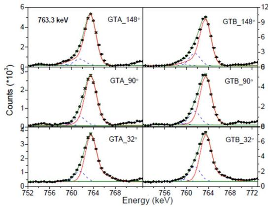
Figure 3. (Color online) Lineshapes of the 763.3 keV  $\gamma$ -transition decaying from the state  $15/2^+$  for the Gating on transition above (GTA) and Gating on transition below (GTB) analyses in DSAM. The fitting in red is the DSAM lineshape, in blue (dashed) is the contaminant peak, and in black is the overall profile.
