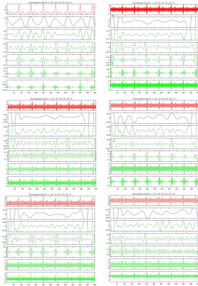
Figure 3. **Top left corner to the right:** ECG signal analysis results with the RSWT with different  $c_q(n)$  for  $q = 1, 2, 3, 4, 5, 6$ . For  $q = 1$  it is the usual wavelet transform.
