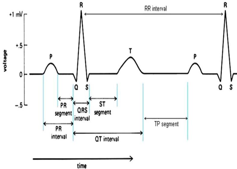
Figure 1. A typical one cycle ECG signal with intervals and segments.
