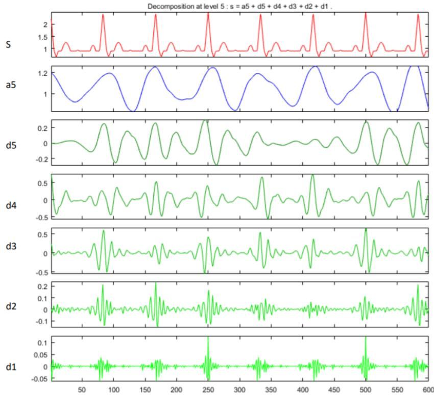
Figure 2. Original signal  $S$ , details  $d1$ – $d5$  and the approximation  $a5$  under the wavelet transform.
