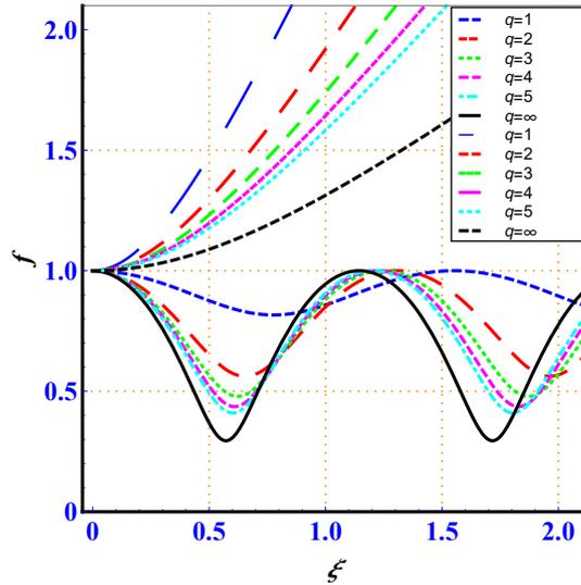
Figure 4. Dependence of beam-width parameter  $f$  with the normalised distance of propagation  $\xi$  for different values of  $q$  (i.e.  $q = 1, 2, 3, 4, 5$  and  $\infty$ ), ( $\rho = 5, p = 2$ , Self-Focusing) and ( $\rho = 1, p = 2$ , Defocusing).
