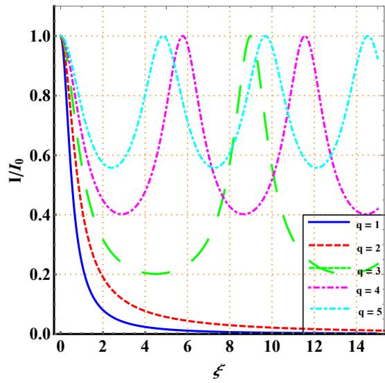
Figure 2. Normalized intensity distribution of  $q$ -Gaussian laser beams for various values of  $q$  ( i.e.  $q = 1, 2, 3, 4, 5$  ) after the  $q$ -Gaussian laser beam entered into the plasma medium.
